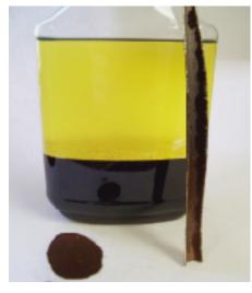
The photograph (left) shows some of the types of ethanol damage encountered in the form of rust taken from the top of an injector tip, a rusted fuel rail and a jar of phase separated fuel.
